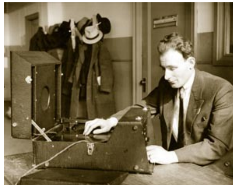
First 33 1/3 rpm Talking Book machine. Picture taken from AFB website.
